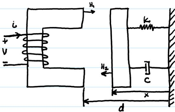
Ampere's law:  $H_1(d-x) + H_2(d-x) = Ni$
